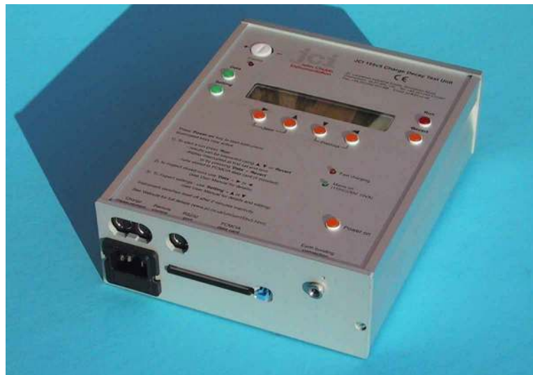
JCI 155v5 Charge Decay Test Unit
