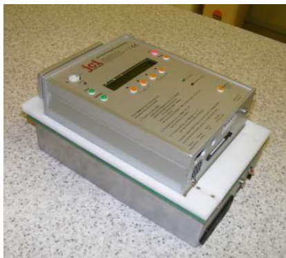
JCI155v5 located on top of the JCI176 sample support
