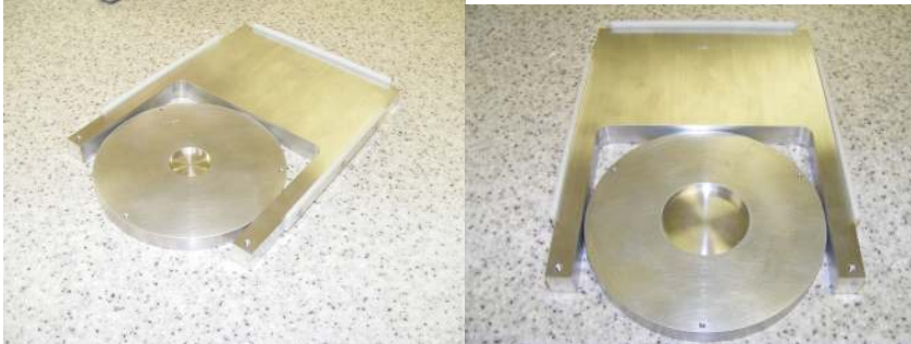
Optional JCI170 powder sample support shown sitting within a JCI172 support for use with the JCI155v5 unit.. Reversal of the JCI170 disc presents a larger or smaller sample test area to the JCI155.
