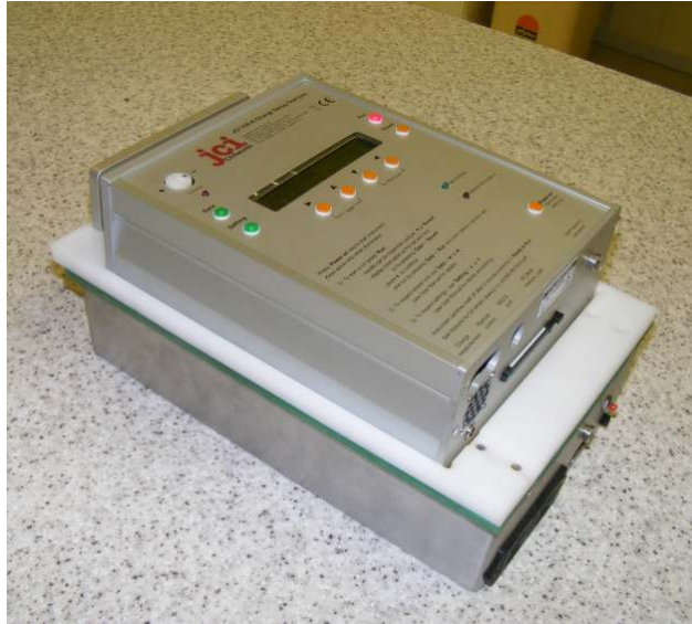
JCI 155v5 on JCI 176 Charge Measuring Sample Support
