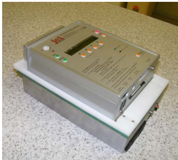
JCI 155v5 shown mounted on top of the JCI176 sample support (suitable for textiles/synthetics/plastics/paper etc material tests but can also be used for testing powder materials when a JCI173 is fitted within the JCI176)
