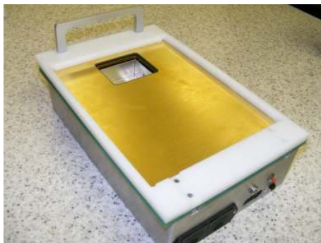
JCI 176 - sample support (textiles/synthetics /plastics/paper etc material tests)
