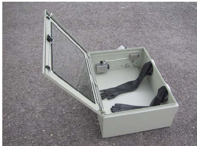
Inside of JCI 191 Controlled Humidity Test Chamber
