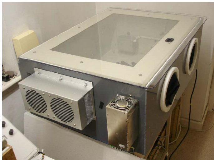
JCI 191C showing power supply and thermoelectric cooler units and overall thermal insulation Controlled Humidity Test Chamber
