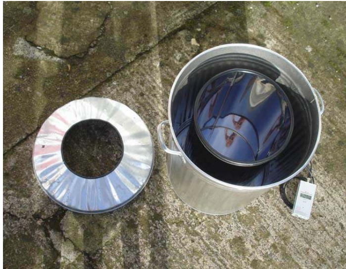
JCI 247 with top cover shield off to show pail
