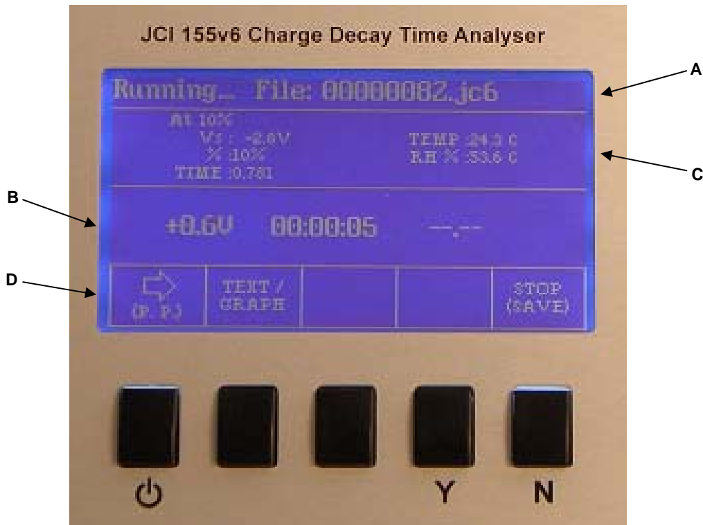
Figure 17: JCI 155v6 Typical Running Screen
