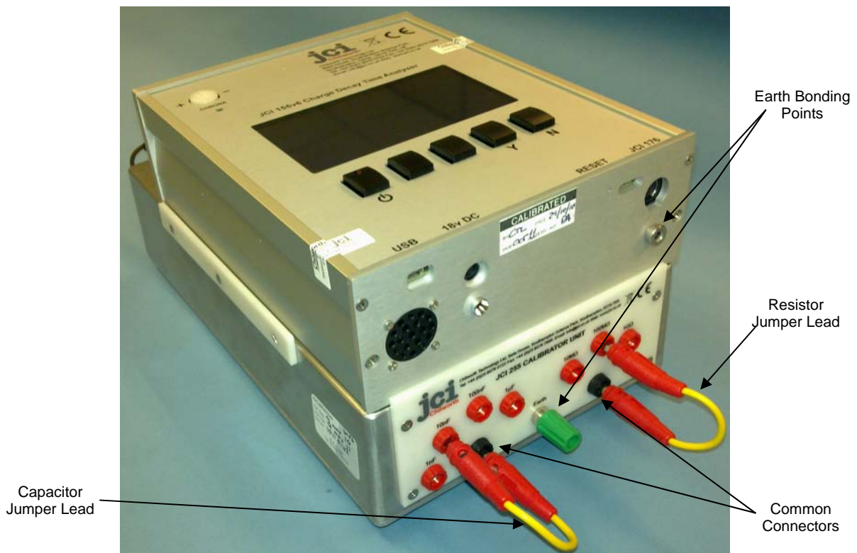
Figure 3: JCI 155v6 Charge Decay Analyser Positioned on the JCI 255 Calibrator Unit
